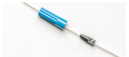
3 - Insert Cable into 0.9 mm Tail Cover
